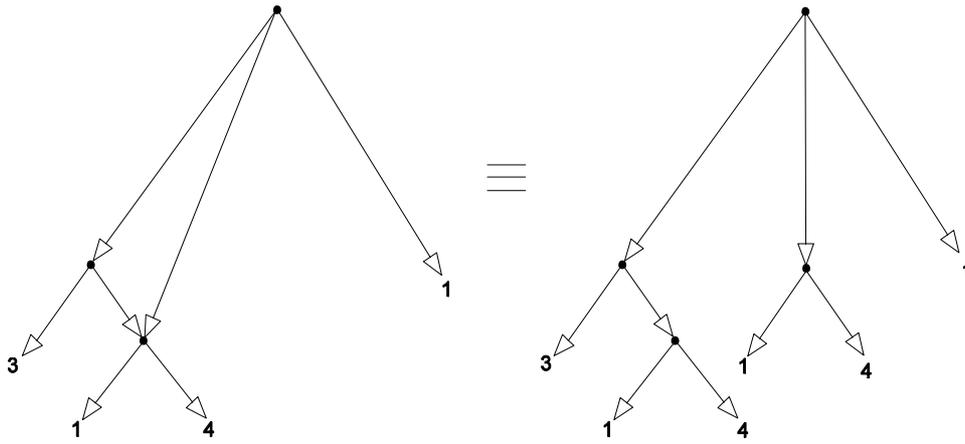
Figure 12: Expansion of a DAG to an Equivalent Out-tree
